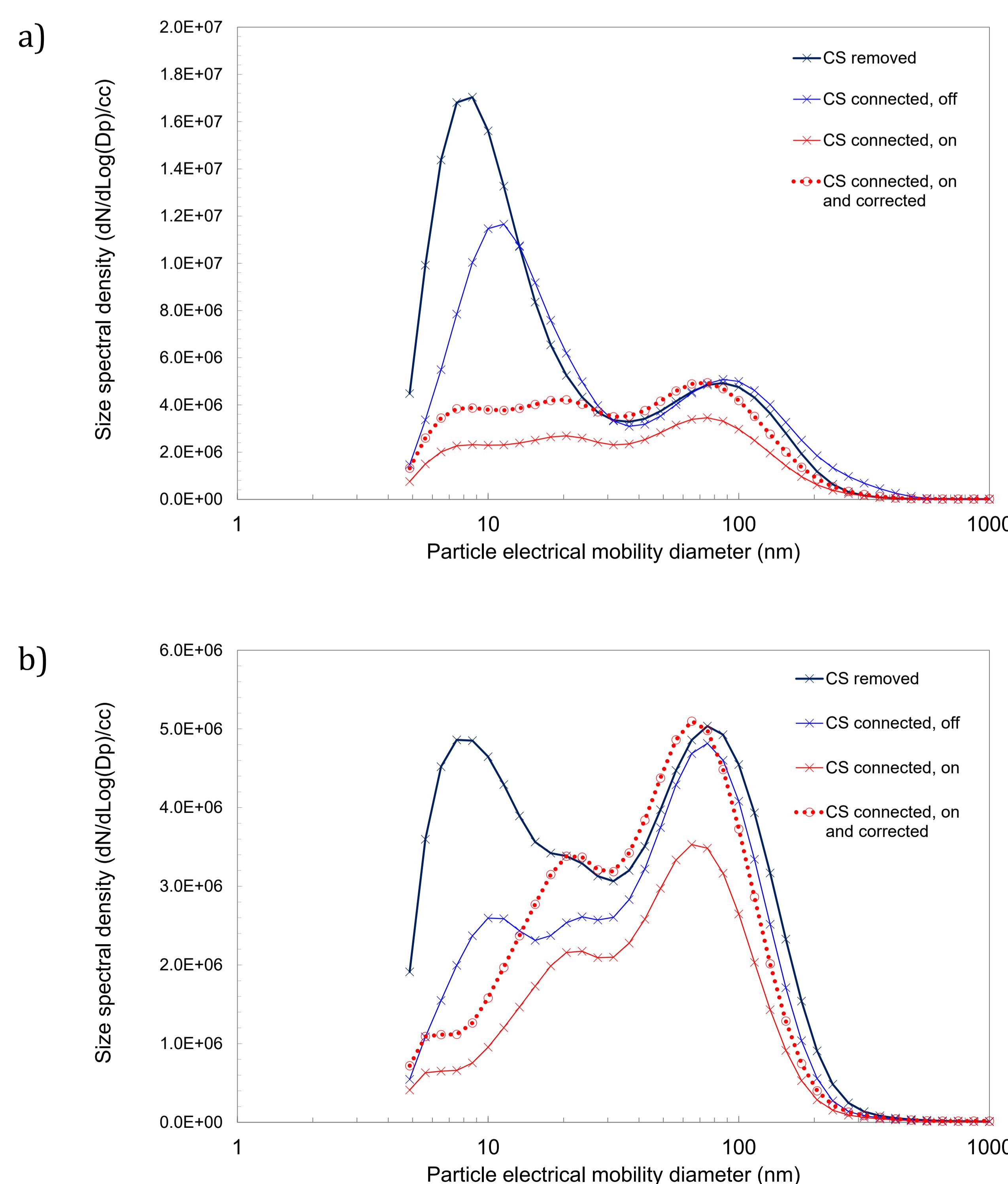
Figure 1: DMS spectra obtained upstream of the turbocharger, with and without a catalytic stripper (CS) in the sample line, a) averaged over the entire cycle and b) averaged over the extra high speed section only.
