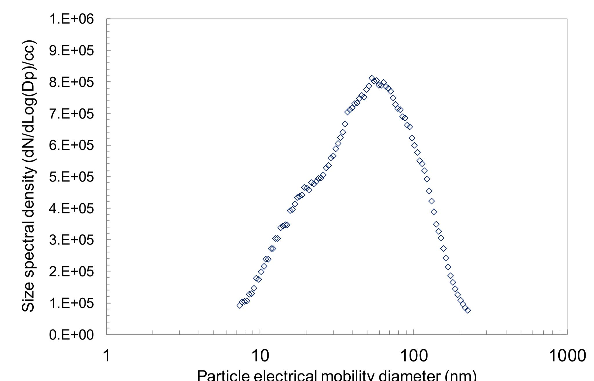
Figure 2: Number size distribution of exhaust particles sampled from the dilution tunnel measured with the SMPS.
