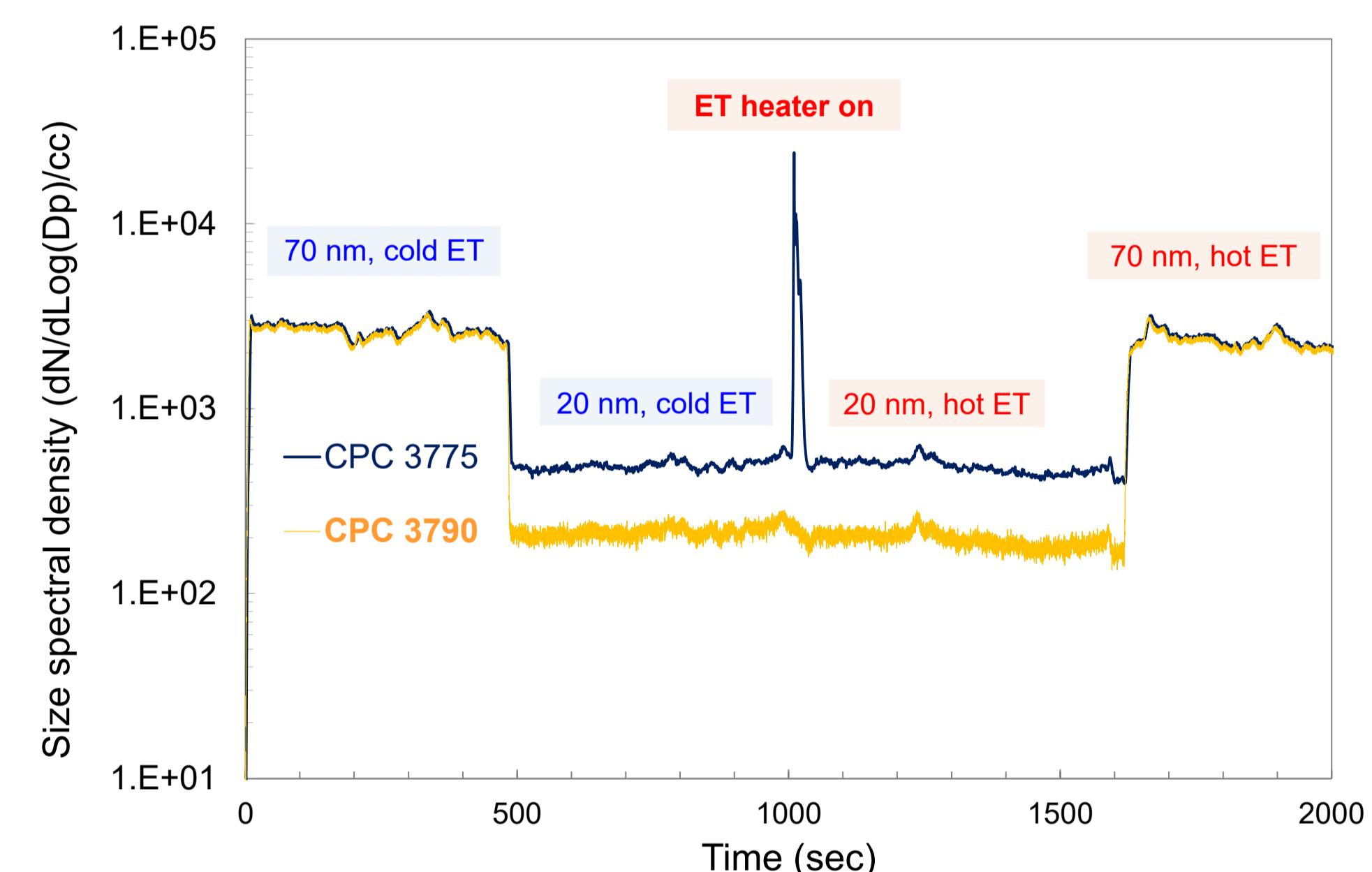
Figure 3: CPC logs while DMA-classified 20nm and 70nm particles are alternately directed through a cold then hot (300°C) ET. The 3775 has a lower cutpoint size (4nm vs 23nm for the 3790) and detects small nucleated particles originating from volatile contaminants within the ET that come off when its heater is activated (reaching setpoint within 30 sec).
