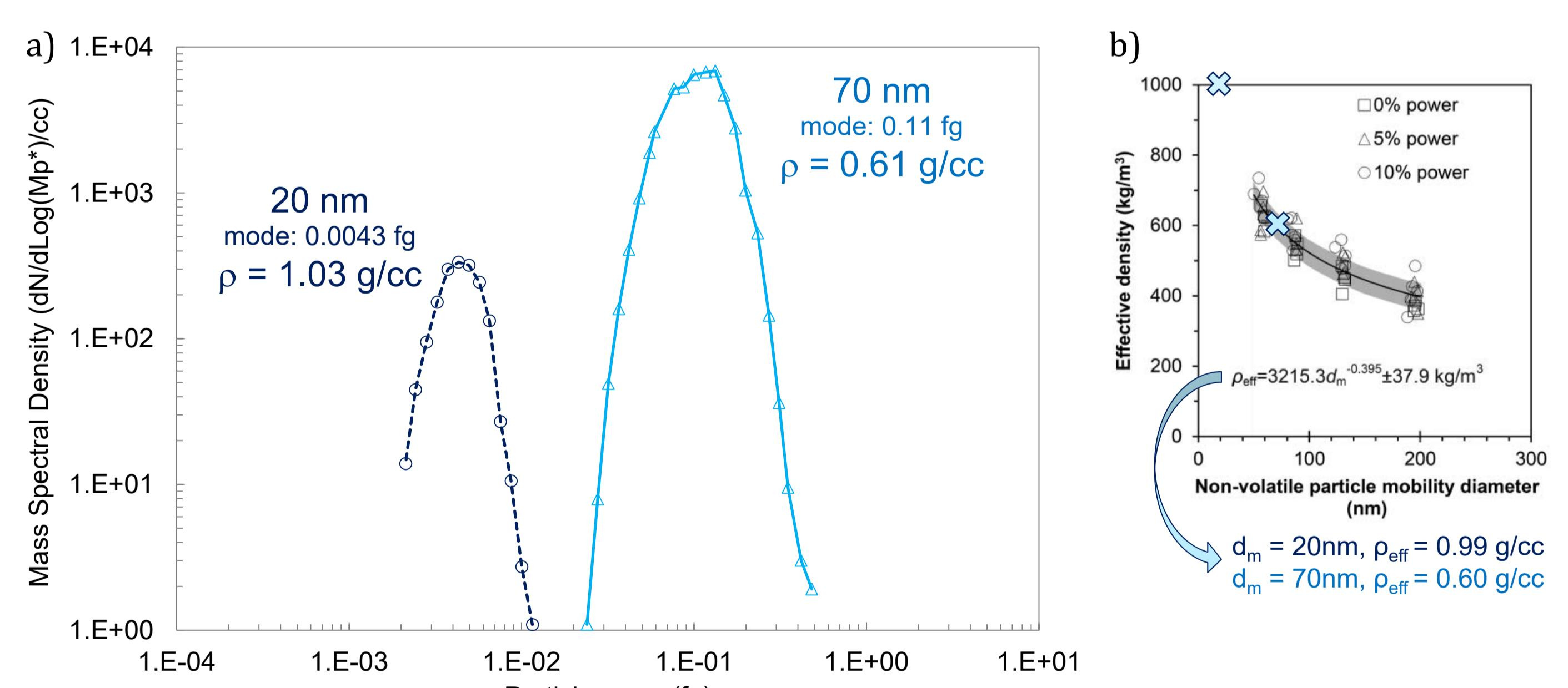
Figure 4: a) CPMA scans of DMA-classified particles taken from the peaks of the modes that appear in the solid particle spectra and b) the effective density values that emerge (blue crosses) plotted with GDI soot data obtained by Momenimovahed & Olfert (2015) who also used the DMA and CPMA in tandem
